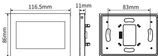
Figure 6. Dimensions - Front View Figure 7. Side View Figure 8. Back View
